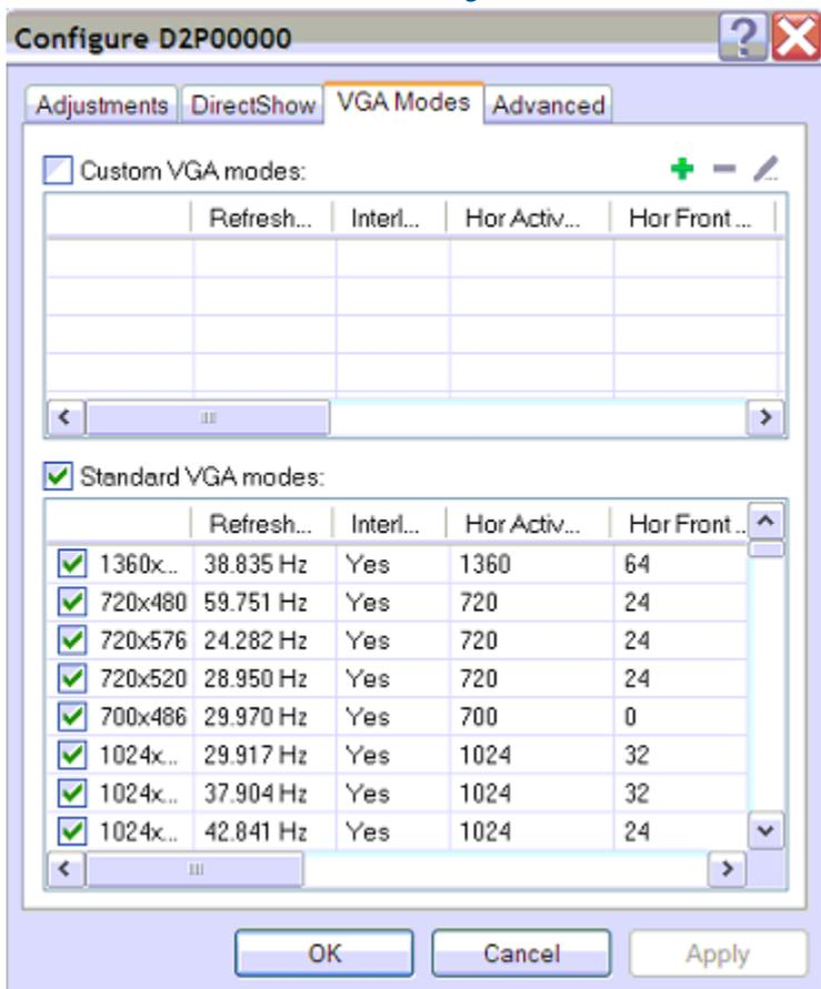
Use this tab to select the standard VGA modes that are used during image capturing.
