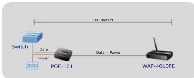
*The IEEE 802.3af Injector and Splitter installation:*
