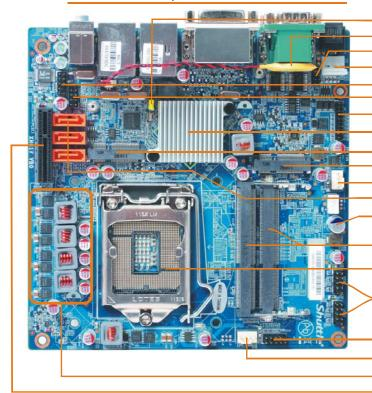
Clear CMOS jumper CMOS battery COM port voltage jumper 19VDC power connector Audio header (front) USB 2.0 header (front) TPM/LPC header Intel H61 chipset
