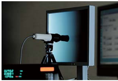
Each monitor adjusted individually at the factory. (For illustrative purposes only. Actual adjustment is performed in a darkroom.)
