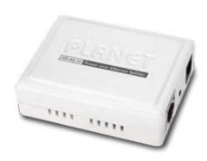
For the cost saving and power management purpose, the PLANET POE-151S is the ideal **IEEE 802.3af Power over Ethernet** device that splits the 48V DC over the Ethernet cable into **5V/12V DC power output**. When working with the IEEE 802.3af power source equipment (PSE), the POE-151S frees the device deployment from restrictions of power outlet locations, which eliminates the costs for additional AC wiring and reduces the installation time.
