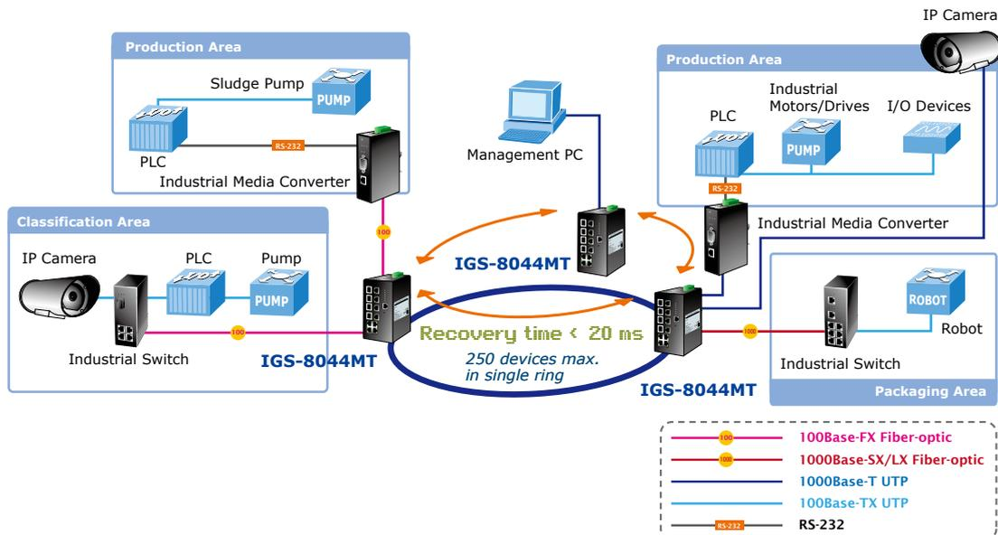
*Coupling Ring – Connection redundant with different area applications*
