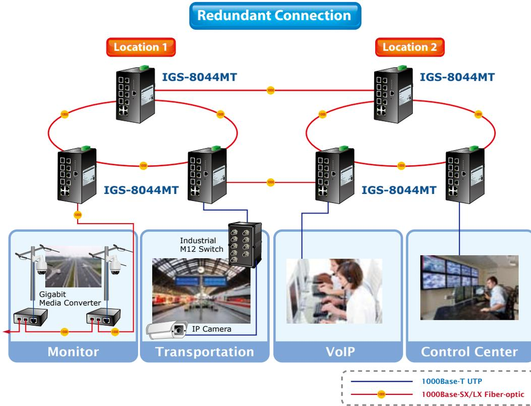
*Dual Homing Ring – Connection redundant with RSTP application*
