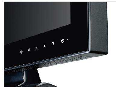
Durable, long-lasting touch sensor controls won't wear out like mechanical buttons
