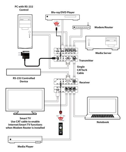
Note: The LAN1, LAN2 and LAN3 connections can be used either on its own as a small network or to extend a larger network. In this example a media player, notebook computer and Smart TV in a remote zone can be connected via a single CAT cable back to a modem/router and media server in another zone with all devices connected to the ports being able to connect to each other.
