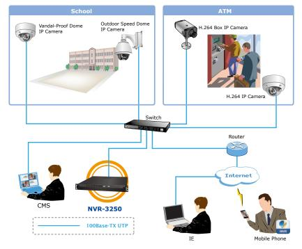
The NVR-3250 enables the administrators to simultaneously monitor the multisite surveillance up to 1024 channels\* via its bundled CMS software, multi-monitor and E-Map functions.
