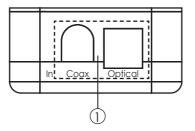
Coax/Optical input: Connect the Coax/Optical inputs into the Coaxial/Optical audio source such as DVD/Blu-ray player or Set Top Box.
