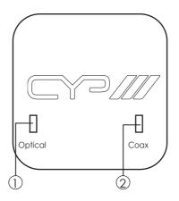
Optical/Coax input LED: The LED light will illuminate according to the fall of input selection switch. The right side LED represent Optical input and the left side LED represent Coaxial input.
