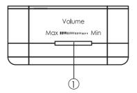
①. Headphone Volume: Adjust the output headphone volume by turning to right or left from small to maximum sound.
