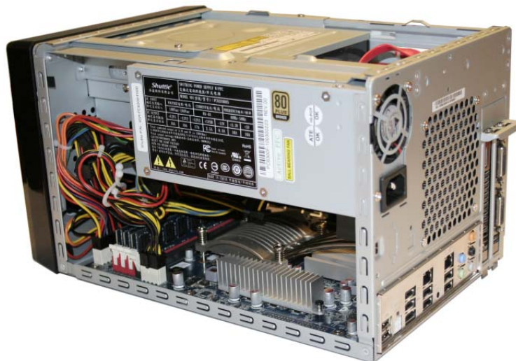
③ Attach the 20-pin ATX and 2x2-pin (or 1x4-pin) power supply plugs to the mainboard.
