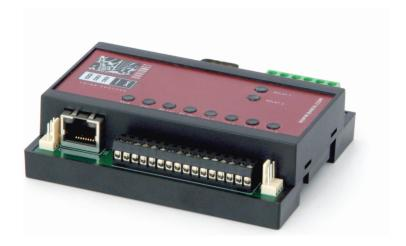
10/100 Mbit Ethernet connection, RS-232 and RS-422/485 serial interfaces, 12 configurable I/Os, 2 relays (240 V, 5 A)
