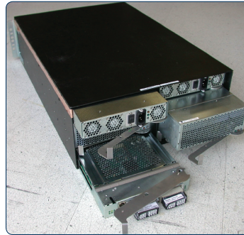
From the rear of the SANbox 9000 chassis module, customer replaceable CPU, power supply, and fan blades are hot-swappable.
